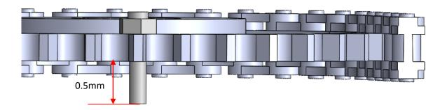
6. Using shortened screws as pins install the rear sprocket mounting plate. Take a note that 2 pins are needed to easily and correctly position the rear sprocket mounting plate.
